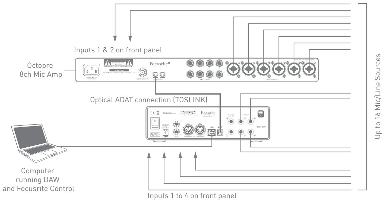
The OctoPre MkII's ADAT output is connected to the Scarlett 18i8's ADAT input with a single TOSLINK optical cable. To synchronise the devices, set the clock source of the OctoPre MKII to **Internal** and that of the Scarlett 18i8 (via Focusrite Control) to **ADAT**.
