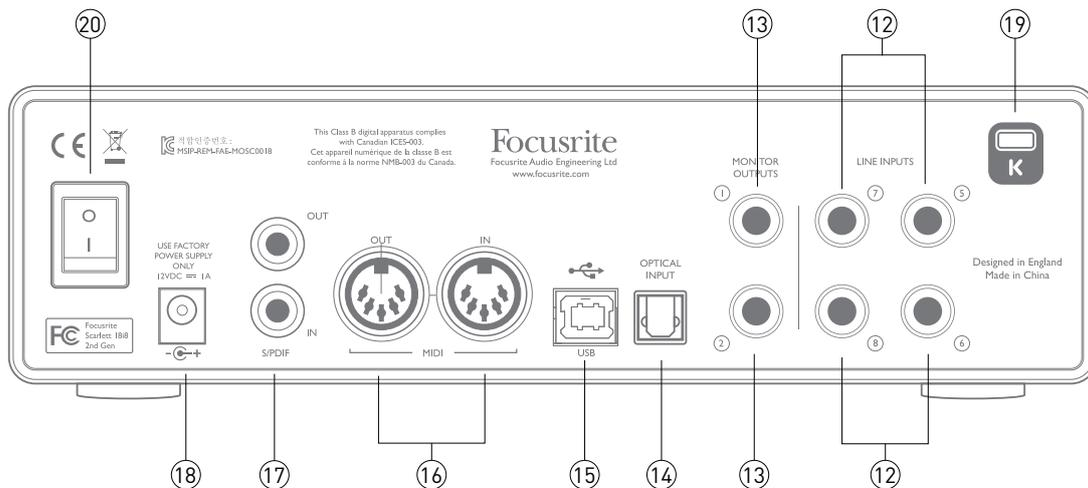
12. **LINE INPUTS 5 to 8** – the inputs are balanced, on ¼” (6.35 mm) jack sockets. Connect line level sources here, using either ¼” TRS (balanced) or TS (unbalanced) jack plugs.
