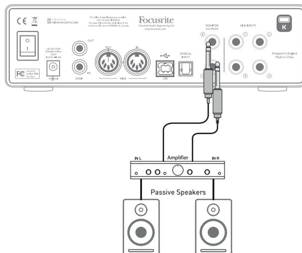
All the line output connectors are 3-pole (TRS) 1/4" (6.35 mm) jack sockets, and are electronically balanced. Typical consumer (hi-fi) amplifiers and small powered monitors will probably have unbalanced inputs, either on phono (RCA) sockets, or via a 3.5 mm 3-pole jack plug intended for direct connection to a computer. In either case, use a suitable connecting cable with jack plugs at one end.
