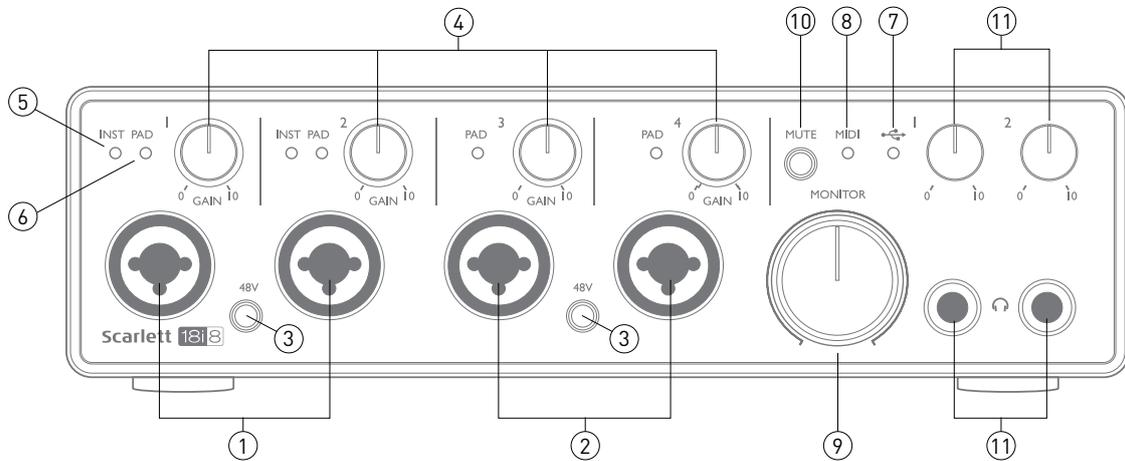
The Front Panel includes input connectors for Mic, Line and Instrument signals, the input gain and monitoring controls, and sockets for headphones.
