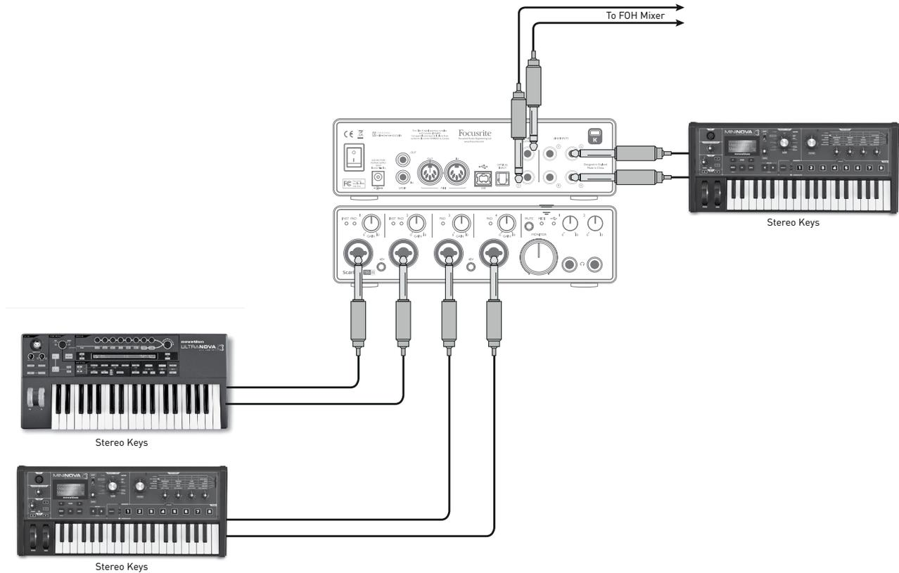
In the example illustrated, three stereo keyboards are connected to the inputs of the Scarlett 18i8; the Monitor Outputs go to the main PA system. The performer can adjust the volume of two of the keyboards against the third from the front panel; he/she can also adjust the overall level of the keyboard mix.
